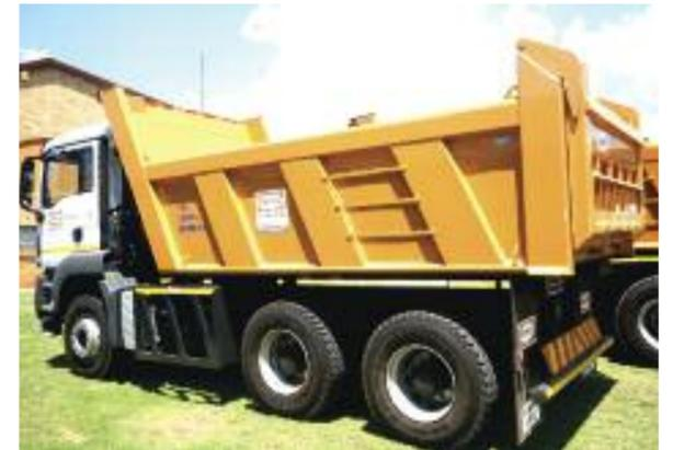
The Renico MAN TGS WW tippers are fitted with 10 cubic-metre tipper bodies from TFM
